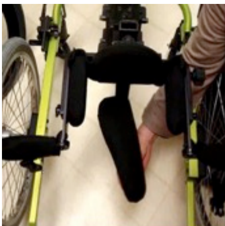
Figure 8: A weight shift mechanism and a swivel seat encourage a more natural gait. (View of the seat and pelvic unit where the child stands and faces forward.)
